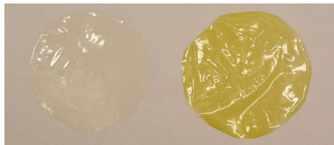
Fig. 2. CS-35G-CD composites conditioned at 75% RH, before (left) and after (right) in contact with carvacrol for three months.
